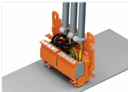
Mounting carrier with strain relief plate mounted vertically on a plate; round cable secured via strain relief lug
