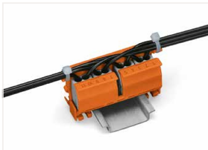
Strain relief via cable ties on the mounting carrier (perpendicular to the connectors' wiring direction); molded marking clamping units
