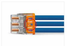
The transparent housing shows if conductors are fully inserted; within the colored base, a clear port shows if the conductor's strip length is correct.
