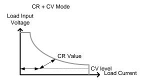
Note that when the source voltage is less than the CV level, no current will flow due to a very high impedance.
