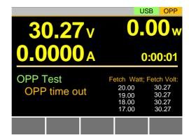
OPP time out will occur if the power supply's OPP fails to trigger. This is determined when the measured voltage is less than Trig V and the measured current is greater than End W.
