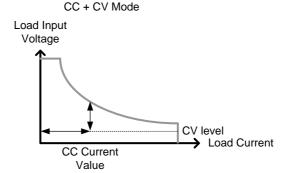
Note that when the source voltage is less than the CV level, no current will flow due to a very high impedance.
