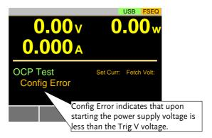
Config Error indicates that the power supply voltage is less than the Trig V voltage setting after the test has started. This can indicate that the power supply output is not on or that the power supply output or Trig V is incorrectly configured.
