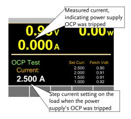
The OCP Test will return the current setting of the last step when the power supply's OCP was tripped.
