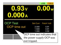
OCP time out will occur if the power supply's OCP fails to trigger. This is determined when the measured voltage is less than Trig V and the measured current is greater than End C.
