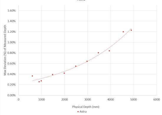
Note: Maximum Deviation has been computed based on the average depth value of the center area of a flat wall positioned at a fixed distance to the camera. The chart is based on Orbbec's internal testing data for your reference.
