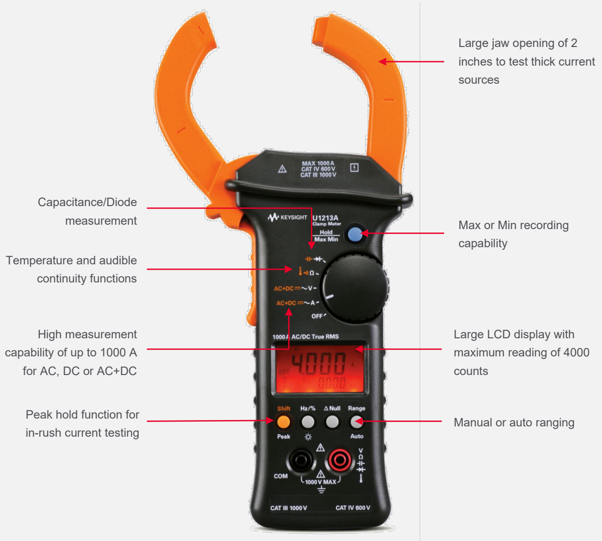
Figure 5. Front view of U1213A handheld clamp meter
