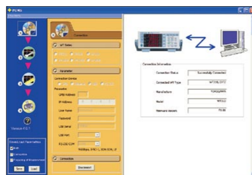
Configuring and Establishing a New Connection between the WT310 and a PC
