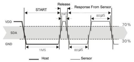
Figure 8 Single Bus Decomposition Timing Diagram
