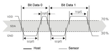
Figure 9 Single Bus Decomposition Sequence Diagram
