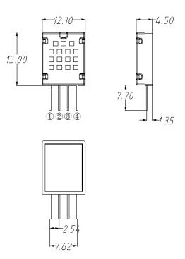
Figure 1 Dimension (Units: mm) Pins 1 VDD 2 SDA 3 GND 4 NC
