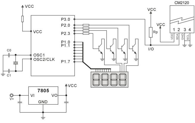
Figure 5 One-Wire Application Circuitry
