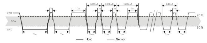
Figure 7 CM2120 Single bus communication timing
