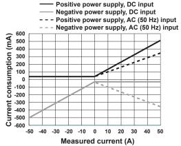
Measured current and current consumption of the 701932/701933 current probe(example of characteristics)
