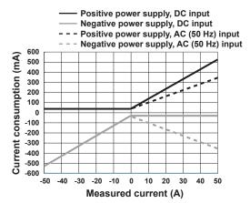
Measured current and current consumption of the 701929 current probe (example of characteristics)
