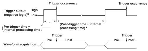
1 High (high level)<sup>3</sup> period: The sum of the pre-trigger time and the internal processing time. The
