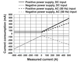
Measured current and current consumption of the 701931 current probe (example of characteristics)
