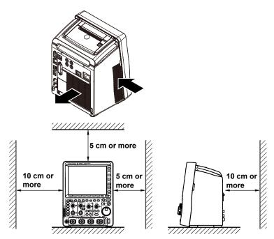
When connecting cables, allow for enough space, above and beyond the space shown in the figure above, to carry out the procedure.
