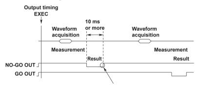
The signal remains low until the instrument is ready to accept the next measurement. If you have specified an action to perform when conditions are true, this time is extended until that action is complete.
