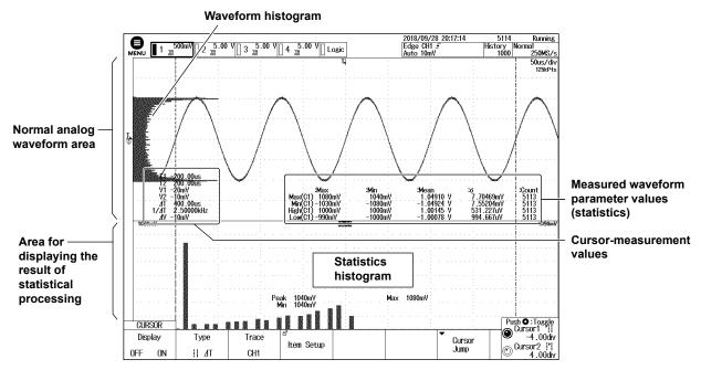
If the setup menu is not displayed, measured waveform parameter values or cursor measurement values are shown in the setup menu display area.
