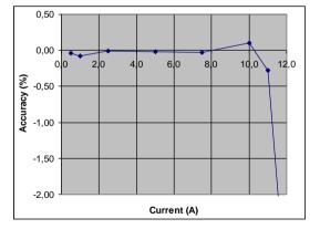
Figure 6: Accuracy vs. current (for 5A range)
