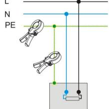
Figure 4: Leakage current measurement – direct method
