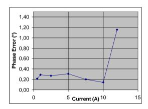
Figure 7: Phase error vs. current (for 5A range)
