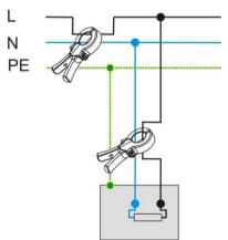
Figure 5: Leakage current measurement – differential method
